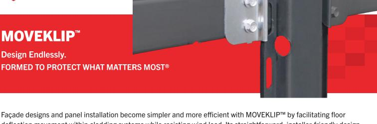
deflection movement within cladding systems while resisting wind load. Its straightforward, installer-friendly design reduces errors and works with PANELRAIL® and various claddings like fiber cement, HPL, and metal panels. Requiring no specialized tools, bolts, or modifications, it simplifies the process and supports virtually unlimited floor movement. With connections that are entirely non-combustible, it ensures reliable fire resistance and safety for every project.
